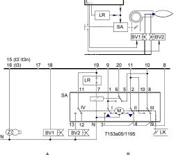
Load control with a 2-position controller. During burner off times, the air damper is closed.
