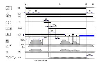
Load control with modulating controller with galvanically separated control contacts for positioning directions «OPEN» and «CLOSE».
